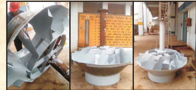
Abrasion & Corrosion Protection of Raw Water Pump Impellers
